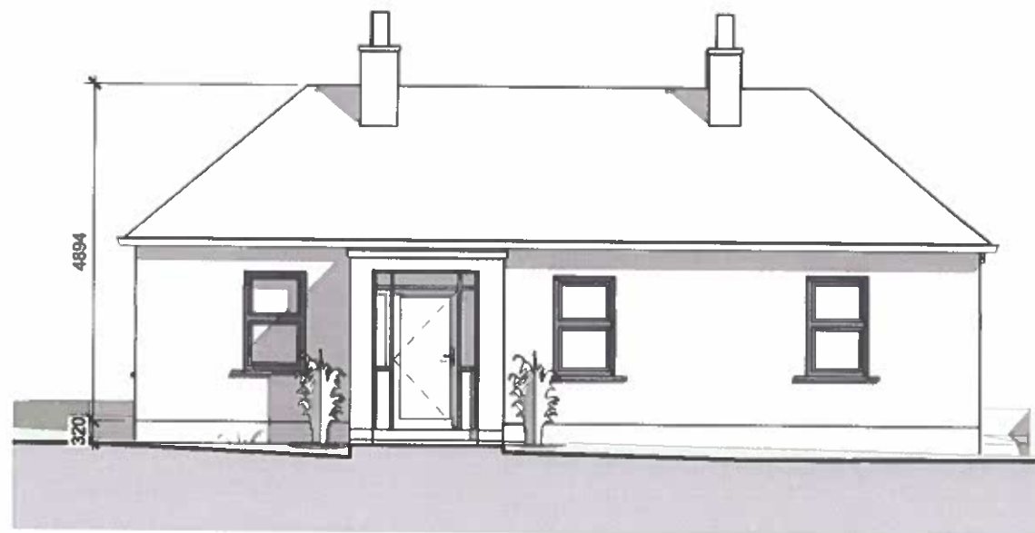
① 01-Front Elevation (E) Existing 1 : 100
