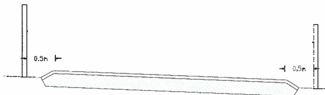
Figure 2 New Farm Roadway Profile (cross section) with camber to one side including fence.
