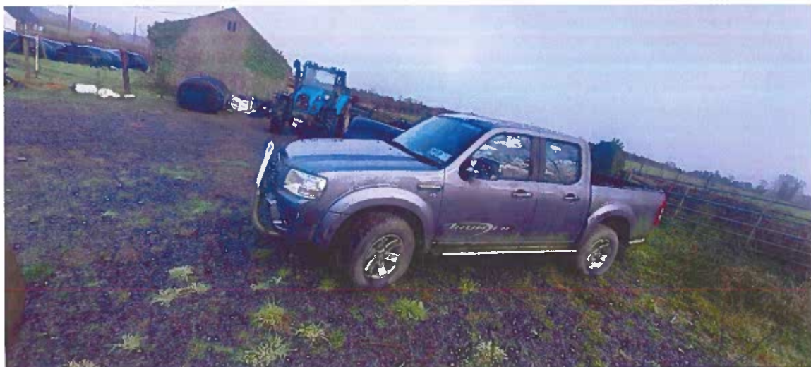
4x4 and Tractor – visible signs of rust on tractor and seals and everything need replacing due to exposure to the elements. Rear Window of Tractor and Side door of tractor have broken due to the seals being damaged by the elements.
