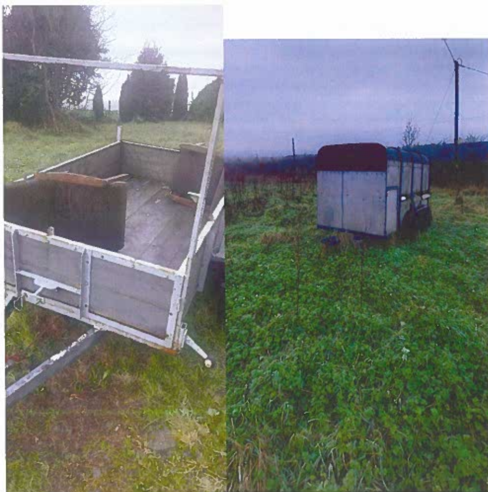
Trailers with timber floors all rotting due to the rain exposure and steel frame starting to rust Cattle trailer sides have rusted, and ball hitch has rusted to the point where it needs replacing
