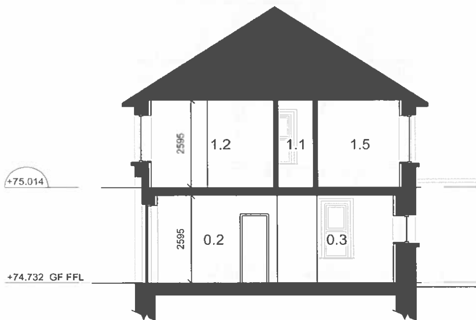
Proposed Section Bb Scale 1:100
