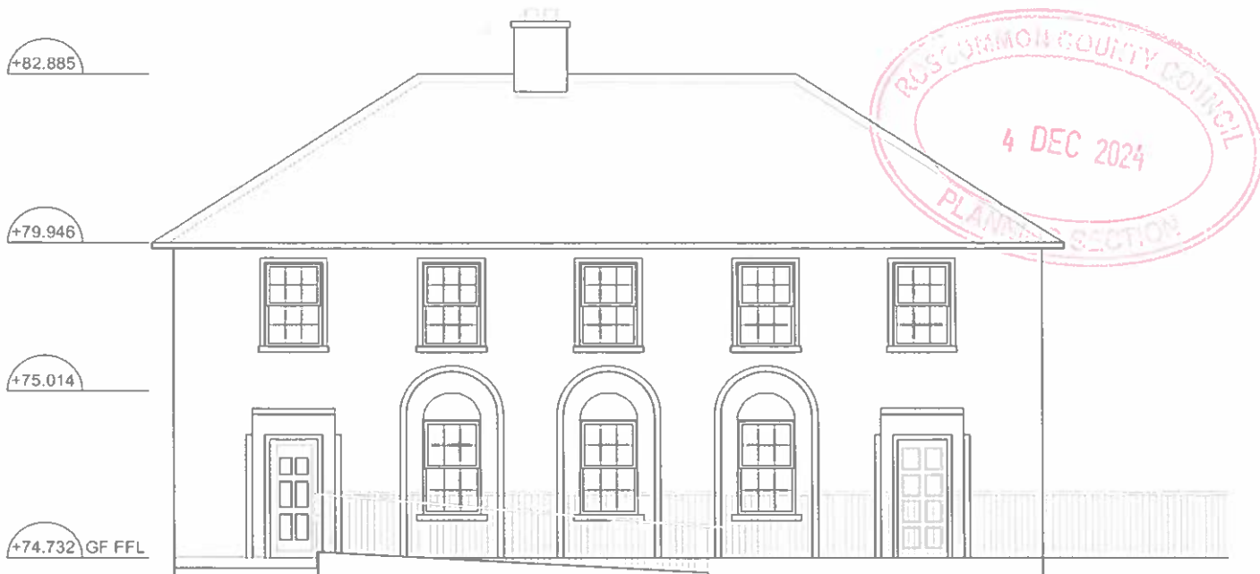
Proposed Front - South-West Elevation Scale 1:100
