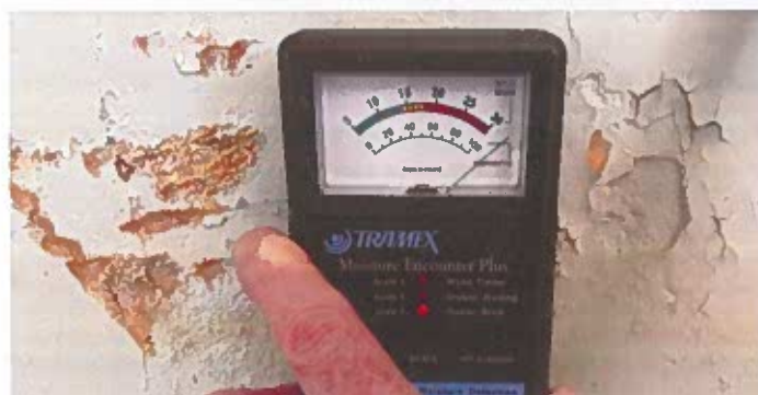
Photos 08d & 08e. There is evidence of high moisture content on the blockwork partition between the living room and bedroom 02. These issues contribute to the cottage been considered derelict and uninhabitable.
