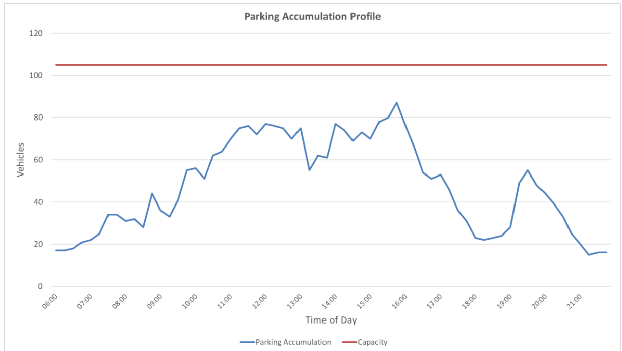
Figure 6.4 Parking Accumulation at The Shop Street Car Park (incl. On-Street Bays)
