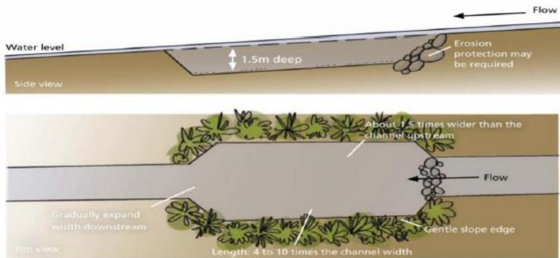
Figure 3. Cross-section and plan views of a sediment trap (Source: https://www.dairynz.co.nz/media/254172/5-9 sediment traps 2012.pdf )
