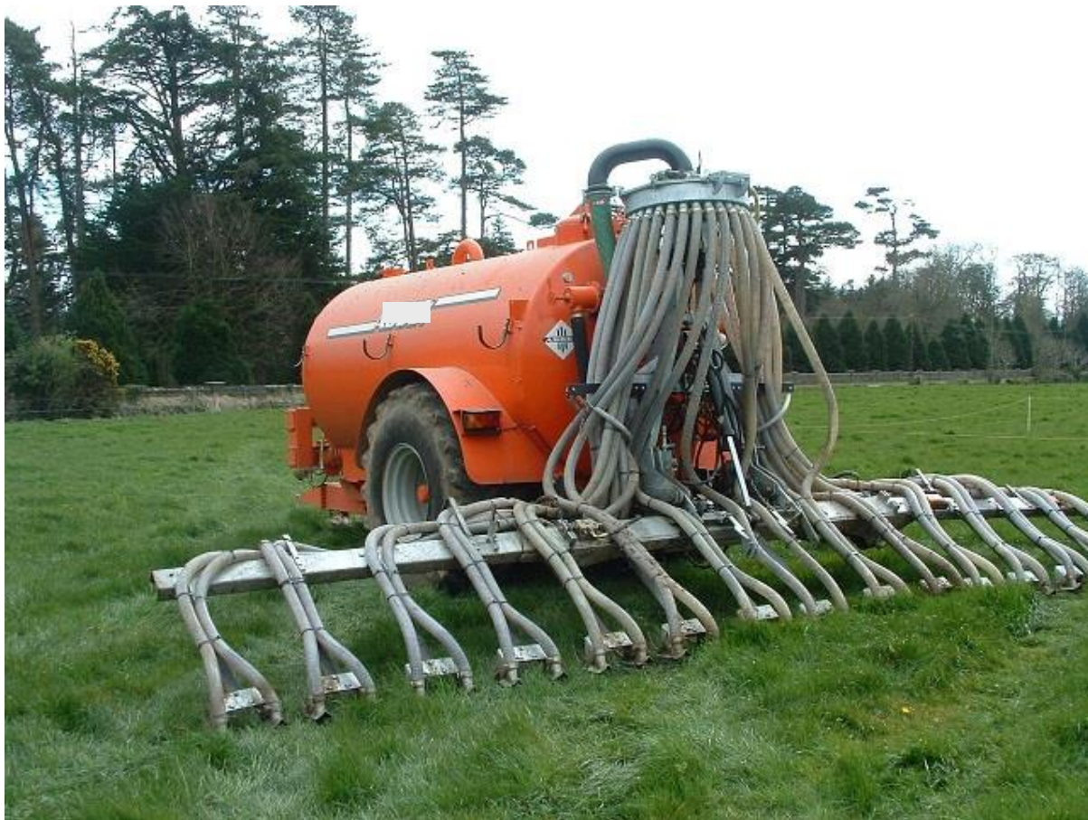
Band spreader/trailing shoe operating off a large vacuum tanker (Photo: Donal Daly).
