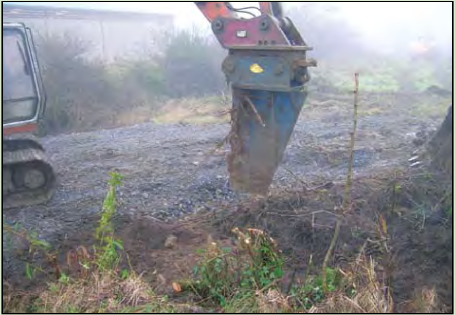
Photo 24: Root cutting attachment
