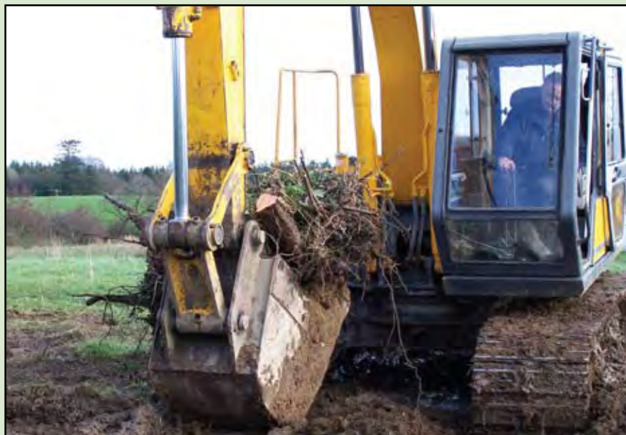
Photo 6: Lifting plants using a non reversible bucket
