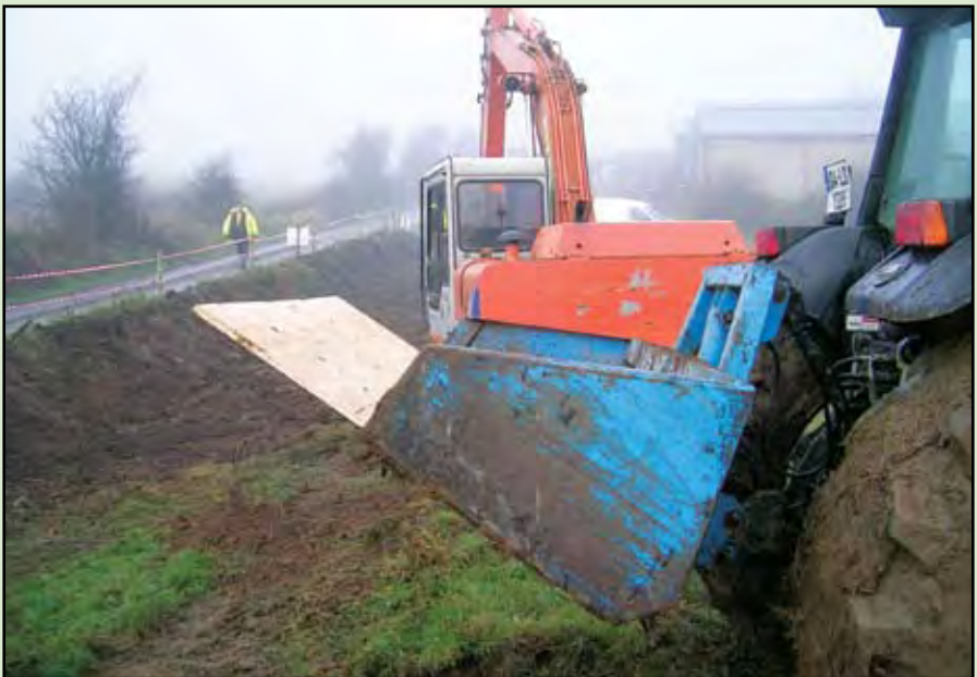
Photo 25: Sheet of plywood used to extend base of transport box
