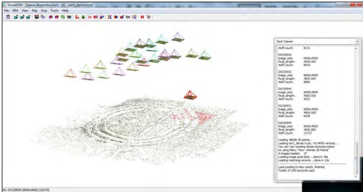
Fig. 2 View of sparse pointcloud output with the solved camera positions
