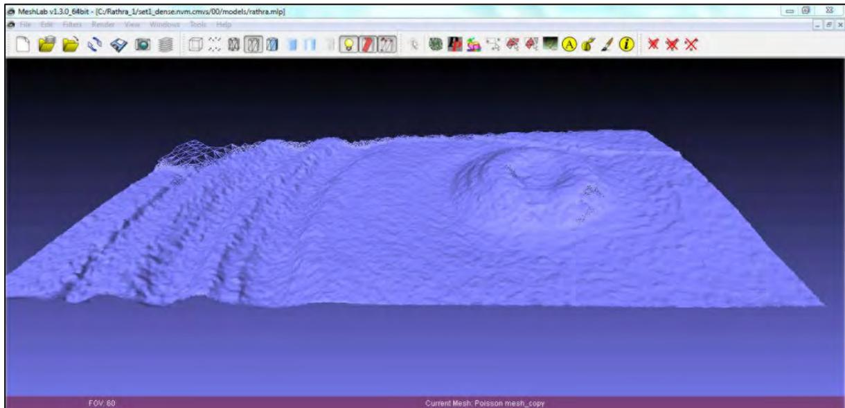
Fig. 4 View of mesh surface modelled from pointcloud data
