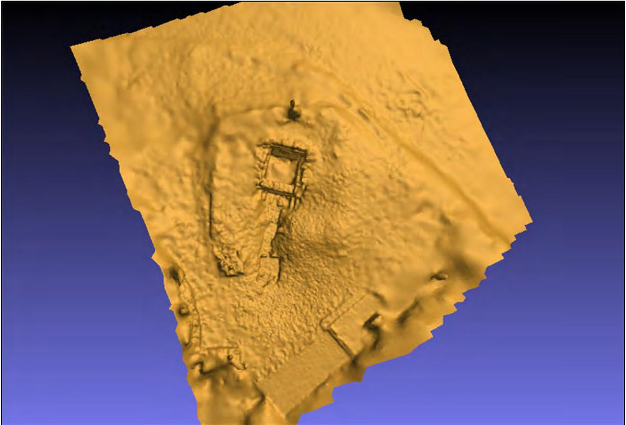
Fig. 7 Aerial view of mesh surface rendered with a 'lattice' shader so that elements of the topography are more clearly visible
