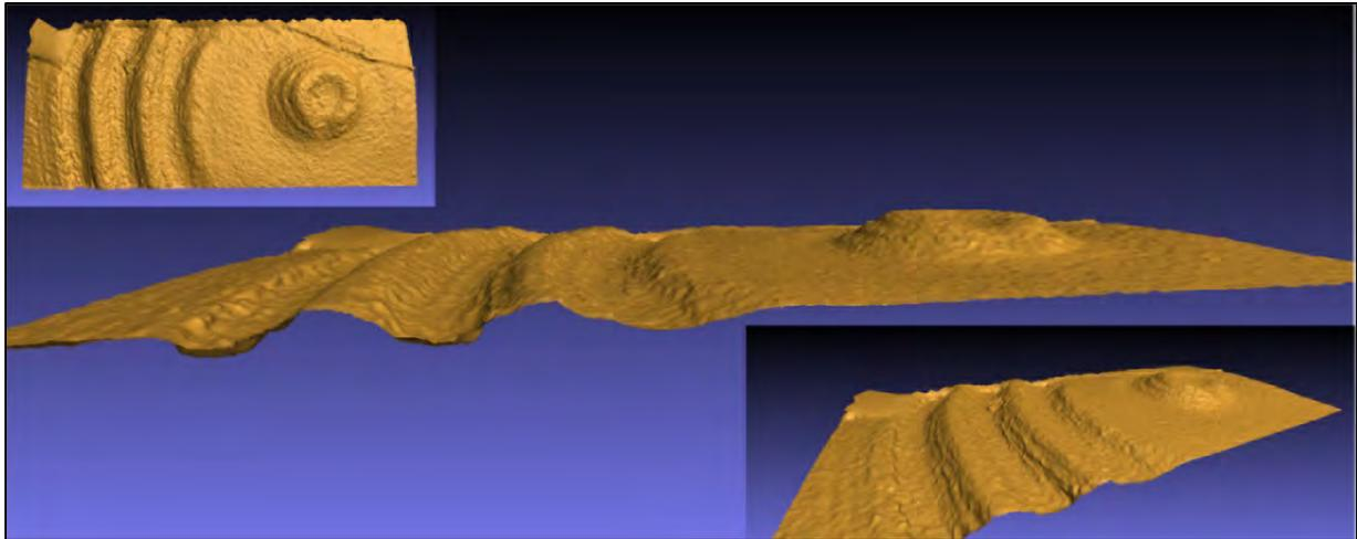
Fig. 13 Sample of the mesh surface derived from pointcloud showing enclosing earthworks and the larger mound barrow at Rathra. This data can also be used to generate profiles through earthworks
