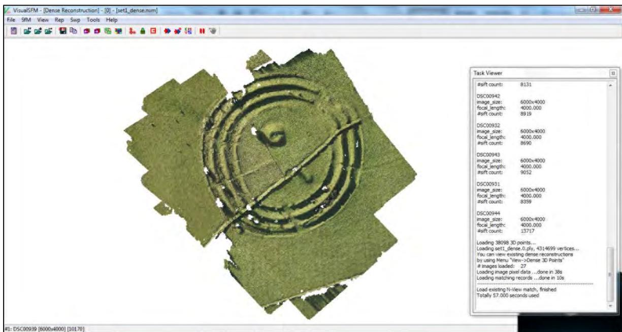
Fig. 3 View of dense pointcloud output. There are 4.3 million individual points in this model (note that each single point has a RGB value). This is **not** a photograph
